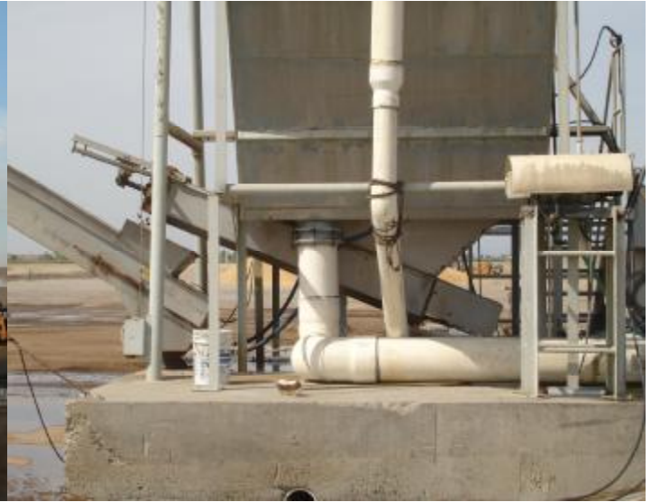
12" x 8' Incline Auger Press (mounted between double 8x12 slope screens)
