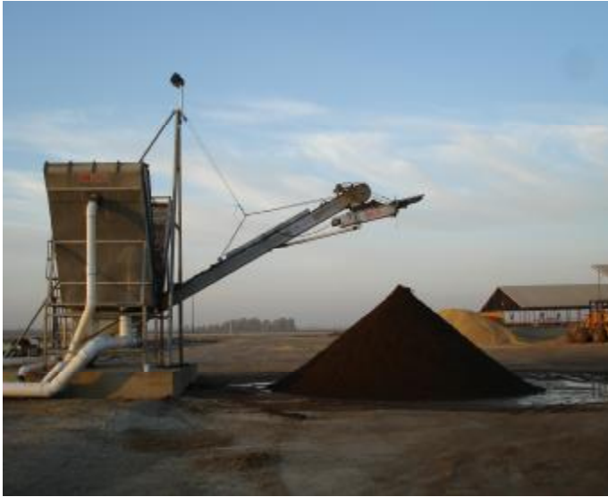
9" x 4' Auger Press (mounted on end of conveyor)
