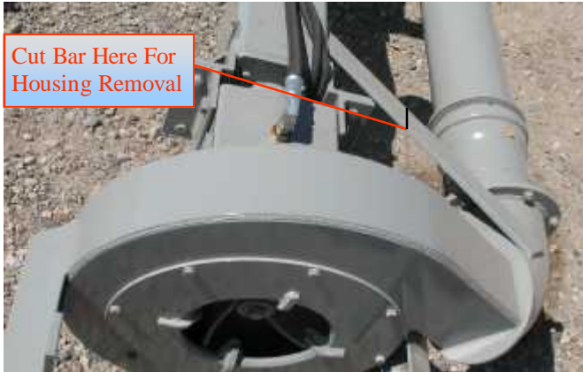
Fig 7 Pump Housing Removal
